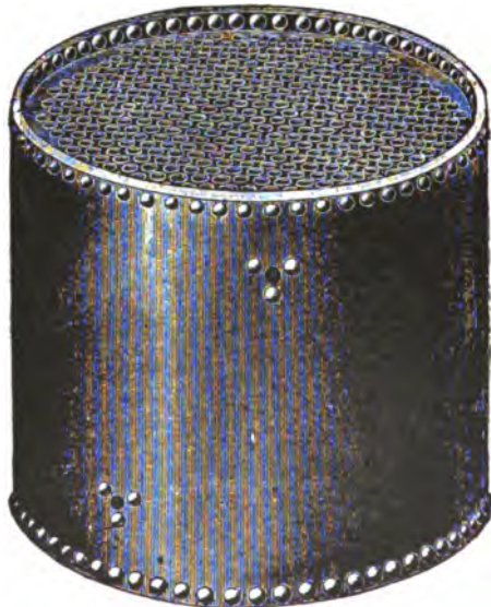
FIG. 147.—Another type of Small Carriage Boiler, showing both tube plates inlanged and riveted to a seamless steel tube.
